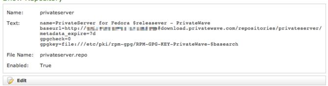
figure 2. Configuration of the single repository
