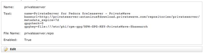
figure 2. Configuration of the single repository
