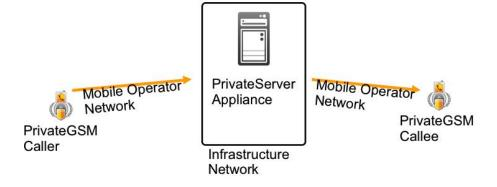
figure 1. A typical network design (semplified)
