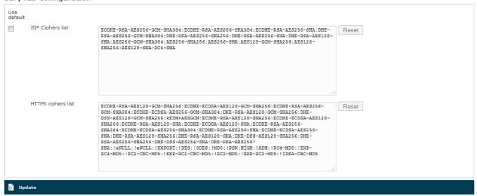
figure 1. Cipher list configuration form
