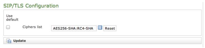
figure 1. Cipher list configuration form
